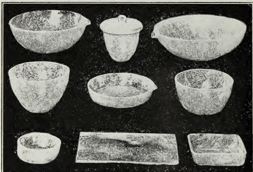
Figure 38.—Laboratory apparatus made of silica.
